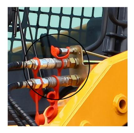
Oil pipe connection: Skid Steer Brush Cutter is equipped with 2 oil pipes, which inlet oil pipe and outlet oil pipe. Connect the tubing to the loader tubing connection.
